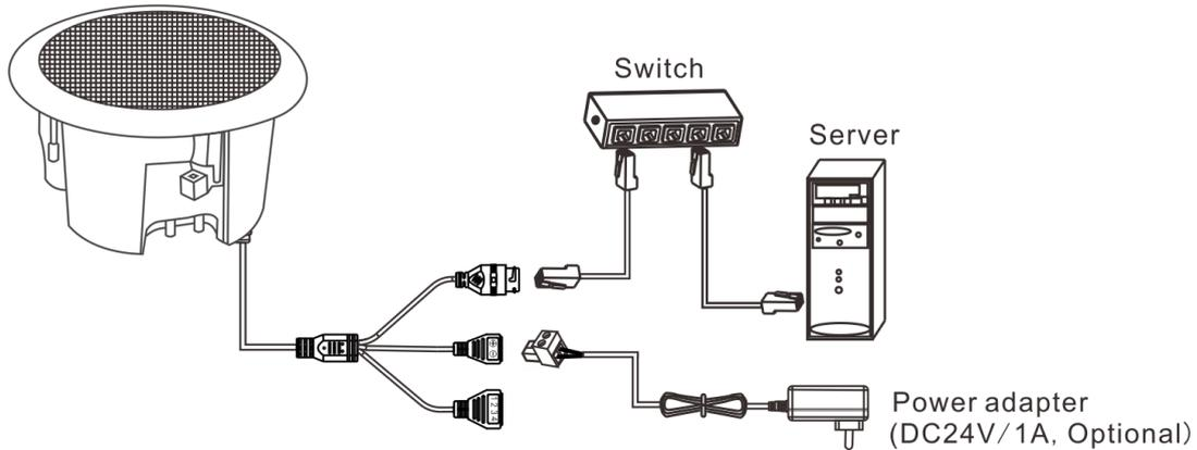
**Note:** POE switcher can not be connected, when using power adapter.
